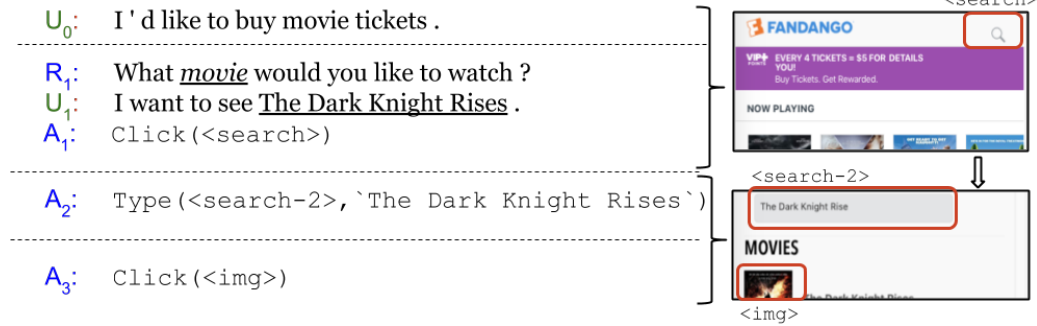
Figure 1: A dialogue with an example web page flow. Detected slot names and values from natural language responses are shown underlined. At time step-2 and time step-3, the system decides to skip interacting with user and continues with acting on the web page ( A_2 and A_3 ).
